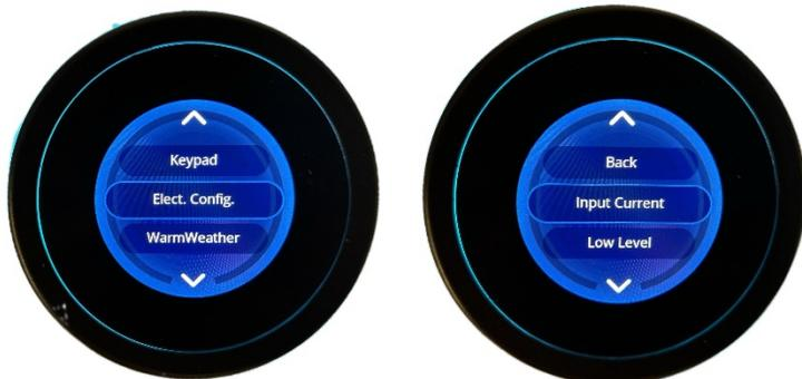
Next, Rotate the dial to scroll thru various **Breaker Settings:**
