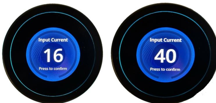
The Breaker Setting should be set at **16** if your **ECO SPA** was set at the factory for **110 Volt** operation.
