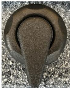
The 3-position **DIVERTER VALVE** allows water to be diverted to a zone of jets, if desired. When the “Pointer Arrow” of the Diverter Valve is centered in the middle (pointed towards the inside of the spa) water flow is directed to all jets. Turning the Pointer Arrow of the Diverter Valve knob all the way to the right or all the way to the left diverts all water flow to a zone of jets on one side of the spa or the other resulting in more robust massage jet action from that zone of jets.
